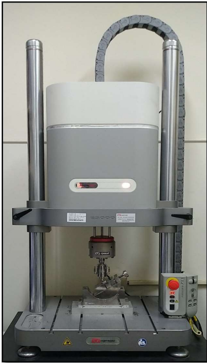
Figure 2: Samples on the test machine Fatigue limit / Maximum endured load at 5,000,000 cycles is 215.82N with maximum bending moment 1187.01 N-mm (conform to CE standard).
