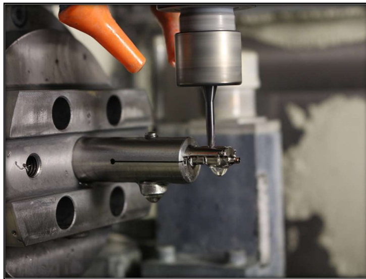
Figure 1: CNC Process (Swiss Type Millturn)
